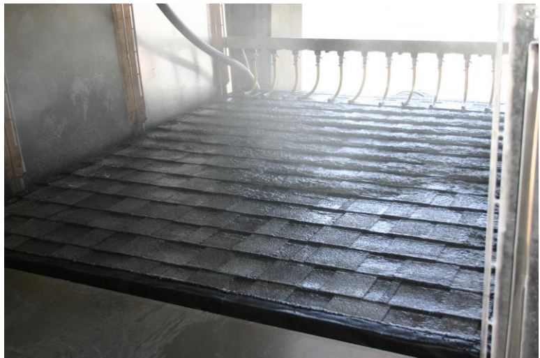
Photo 6 Overview of wind-rain combination B (with extra wind) on test specimen 1 at a slope of 7,5°.
