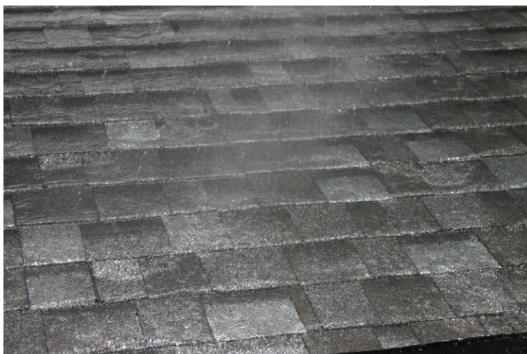
Photo 11 Detail of wind-rain combination B on test specimen 2 at a slope of 15°.
