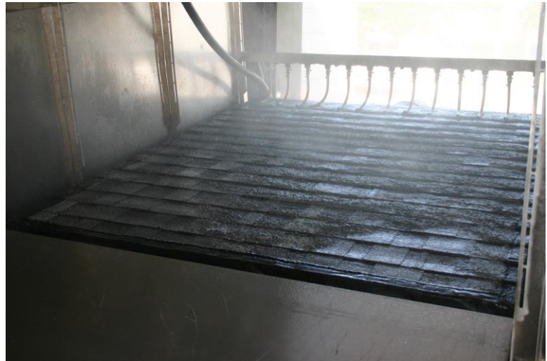
Photo 7 Overview of wind-rain combination B (with extra wind and extra water) on test specimen 1 at a slope of 7,5°.
