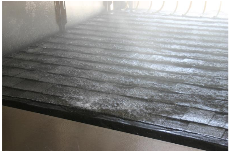
Photo 8 Detail of wind-rain combination B (with extra wind and extra water) on test specimen 1 at a slope of 7,5°.
