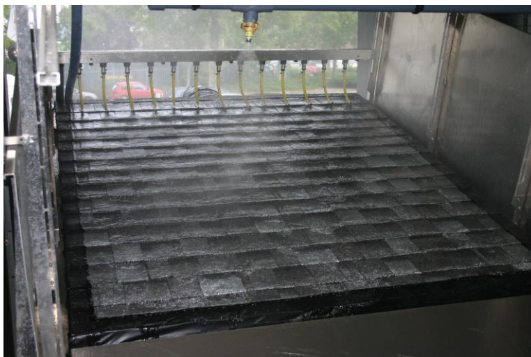
Photo 10 Overview of wind-rain combination B on test specimen 1 at a slope of 15°.
