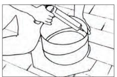
Seal the adjusting seam and the base/collar connection seam on inside with roofing cement. Seal locking clamp holes and all exposed nails with roofing cement.
