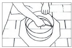
Choose location of turbine from the front page. Center between two rafters and mark hole to be cut.
