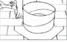
Slide top half of flashing under shingles all the way to the collar. Seal around and secure with the roofing nails at top, sides and bottom.
